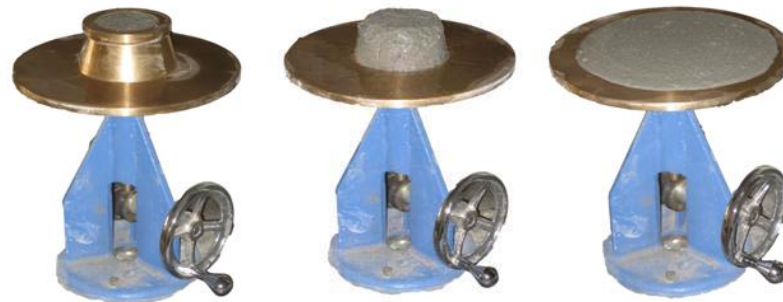
a) Mortar in conical frustum b) Prior to dropping table c) After 25 drops
